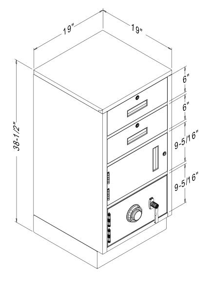
TWO KEY-LOCKING BOX DRAWERS OVER ONE KEY-LOCKING CUPBOARD DOOR OVER ONE 1/4" THICK FRAME LOCKER BEHIND A 1/2" THICK STEEL PLATE DOOR EQUIPPED W/ A GROUP II SPY PROOF MECH. COMBO LOCK.
