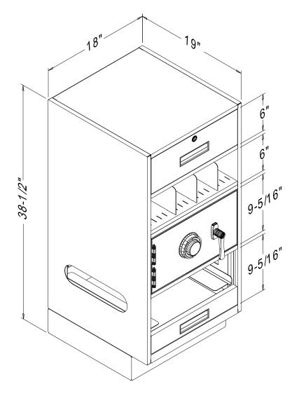
A KEY-LOCKING BOX DRAWER OVER A P-51 FORMS HOLDER W/3 ADJUSTABLE DIVIDERS OVER ONE 1/4" THICK FRAME LOCKER BEHIND A 1/2" THICK STEEL PLATE DOOR EQUIPPED W/ A GROUP II SPY PROOF MECH. COMBO LOCKOVER A **VENTILATED CPU COMPARTMENT** W/ A PULL-OUT CPU SHELF.
