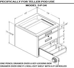
COIN TRAY BEHIND AN 1/8" THICK STEEL PLATE LOCKER DOOR EQUIPPED WITH A GROUP II MECH, COMBO LOCK.
