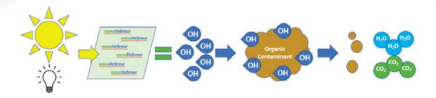
Light triggers the nanoDefense™ Self Cleaning Process which produces Hydroxyl radicals that attack and decompose organic contaminants into water, carbon dioxide, and harmless byproducts
