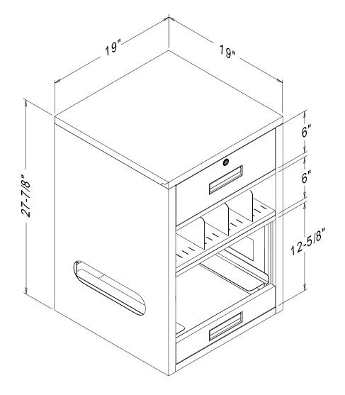
A KEY-LOCKING BOX DRAWER OVER A P-51 FORMS HOLDER W/ 3 ADJUSTABLE DIVIDERS. OVER A VENTILATED CPU COMPARTMENT W/ A PULL-OUT SHELF.
