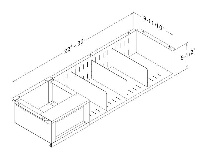
P-52 KNEE-SPACE HOUSING (APRON CASE WITH PIN AND CLIP TRAY), TO BE ADJUSTABLE FROM 22-30"W X 5-1/2"H X 9-11/16"D, INCLUDES PIN AND CLIP TRAY. WITH FLAPS ON EACH END FOR EASY INSTALLATION. INCLUDES THREE ADJUSTABLE PARTITIONS (MODEL P-25).
