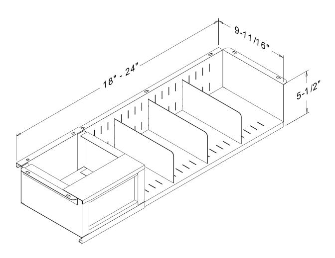
P-24 KNEE-SPACE HOUSING (APRON CASE), TO BE ADJUSTABLE FROM 22-30"W X 5-1/2"H X 9-11/16"D - WITH FLAPS ON EACH END FOR EASY INSTALLATION. INCLUDES THREE ADJUSTABLE PARTITIONS (MODEL P-25).
