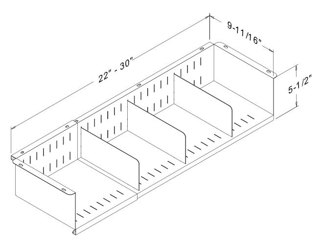
P-24 KNEE-SPACE HOUSING (APRON CASE), TO BE ADJUSTABLE FROM 22-30"W X 5-1/2"H X 9-11/16"D - WITH FLAPS ON EACH END FOR EASY INSTALLATION. INCLUDES THREE ADJUSTABLE PARTITIONS (MODEL P-25).
