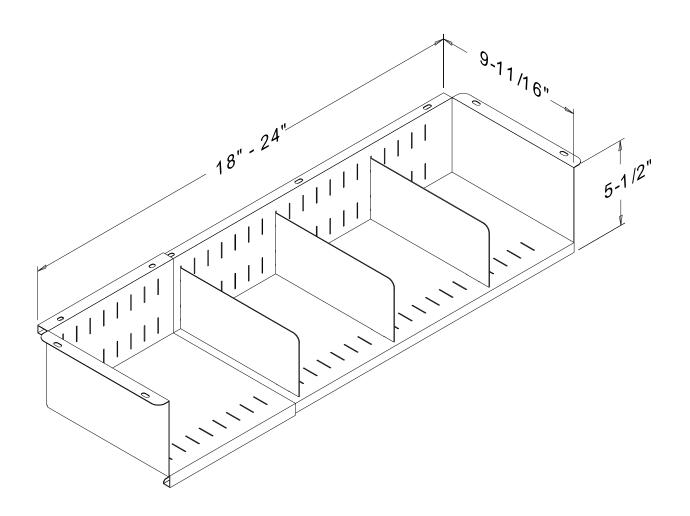
P-24 KNEE-SPACE HOUSING (APRON CASE), TO BE ADJUSTABLE FROM 18-24"W X 5-1/2"H X 9-11/16"D, WITH FLAPS ON EACH END FOR EASY INSTALLATION. INCLUDES THREE ADJUSTABLE PARTITIONS (MODEL P-25).
